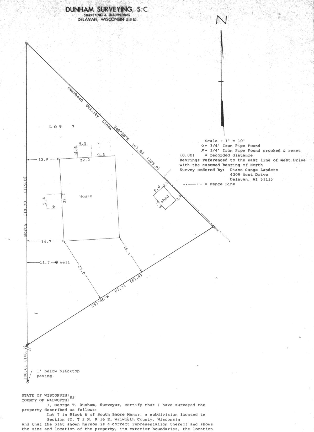
of all visible structures and dimensions of all principal buildings thereon, boundary fences, apparent easements, roadways and visible encroachments, if any, and that I have surveyed the property hereon described, according to the official records, to the best of my knowledge and belief.
